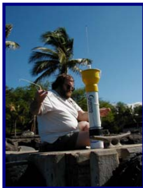
Adam Frankel rigs a sonobuoy for a water test at Kawaihae Harbor
